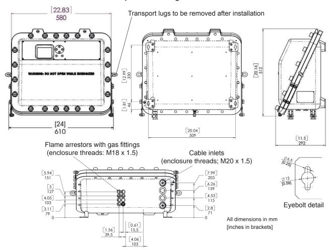
Fig. 2-12: X-STREAM X2FD - Dimensions
